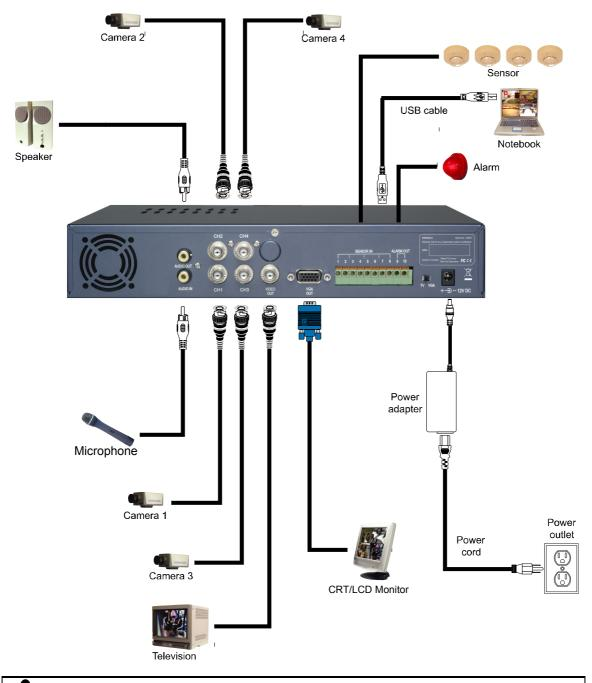
The DVR unit support 2 video output ports and you can only select ONE to output the video either from the VGA OUT or VIDEO OUT.
